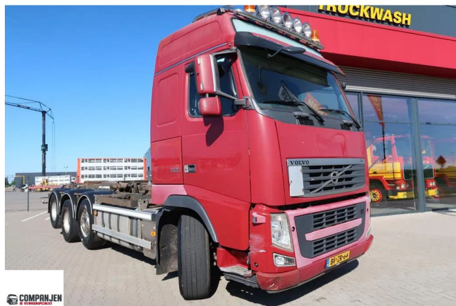
Volvo FH 520 FH - 8x4 R - Ketting systeem
